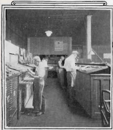
Composing Room showing dust proof cabinets which contain hundreds of different styles of type.
