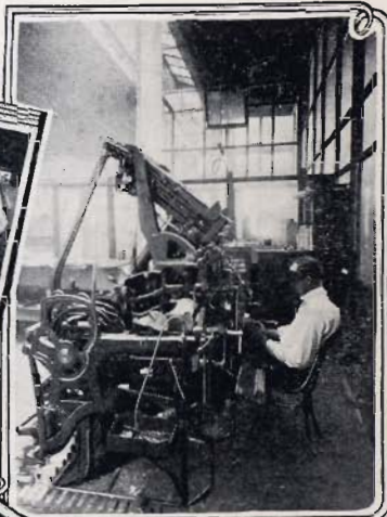
Linotype-Type setting machine which produces a product equal to SK men.
